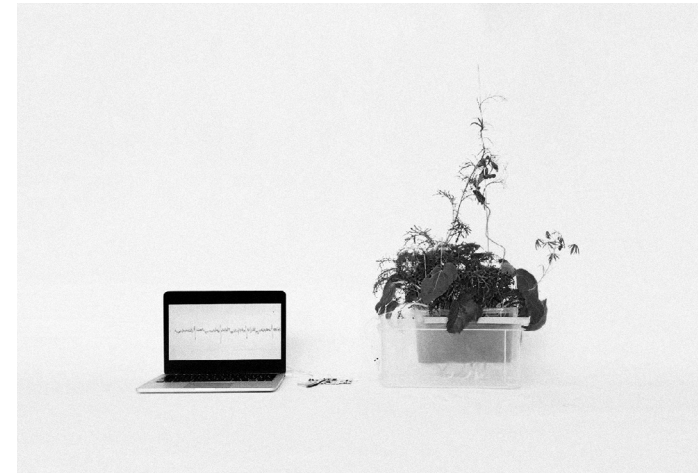
Figure 1: Setup connecting an open hardware electro-myography sensor (EMG) to an assembly of plant-life.
